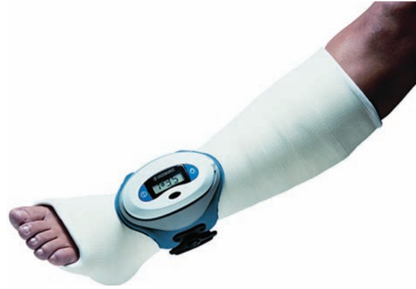
Figure 27•4 PEMF induction of an electric field into a fracture site to promote healing. A non-surgical option for long bone and small bone nonunion and delayed union fractures, the device may be worn over a cast, orthopedic device, of clothing without lessening its effectiveness. (Physiostim™ Model 3202, permission of Orthofix Inc., McKinney, TX)
